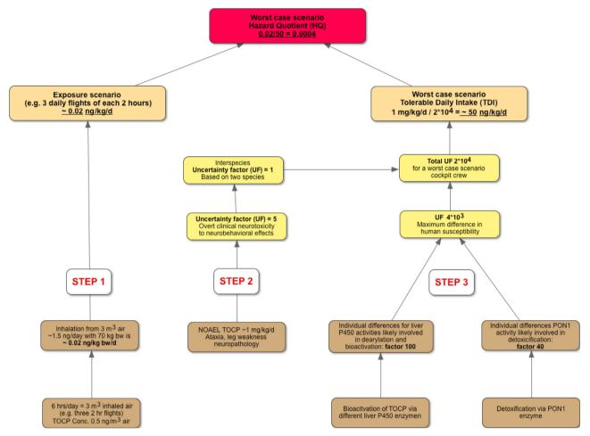
Fig. 2. Schematic presentation of the model that estimates the risk of potential ToCP exposure in KLM B737 airplanes for cockpit crews.
